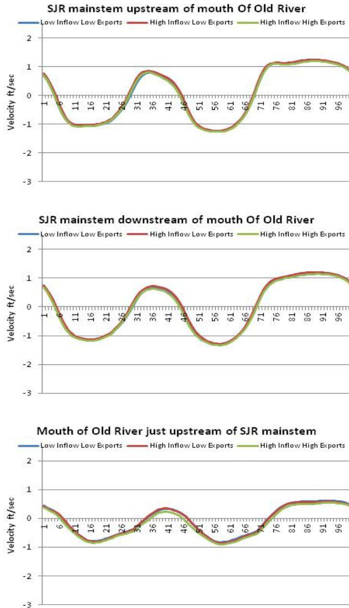
**Figure 3-8. DSM2 Modeled Instantaneous 15-Minute Velocity Versus Time Over a Complete Tidal Cycle (~25 Hours) in Three Channels at the Junction of the San Joaquin River Mainstem and the Mouth of Old River**
